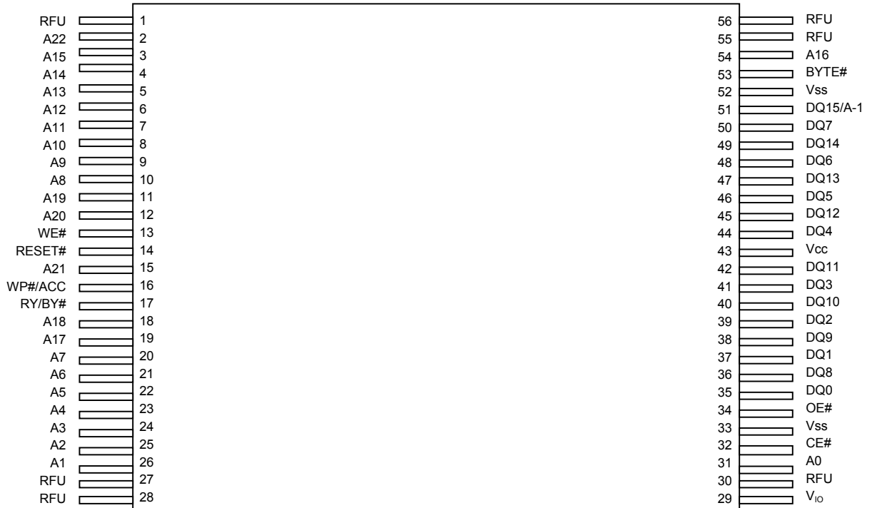
Figure 1. 56-pin Standard TSOP (Top View)
