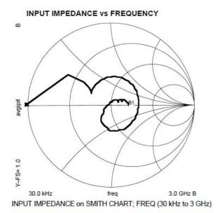
Note: All measurements performed on Hewlett Packard 8753D Network Analyzer (201 sample points, linear scale) in a 50 ohm coplanar waveguide
