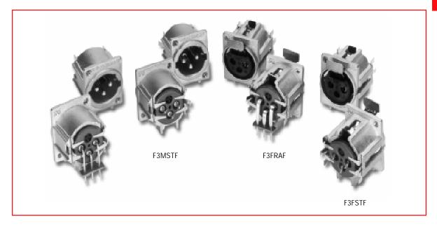
Switchcraft now offers the F Series. Available in male and female, the receptacles can be mounted from the rear of the panel. Features include an all metal housing with a ferrite disk for added EMI/RMI shielding. Both male and female connectors can be mounted vertical or horizontal to the PC board. All connectors have a PC-board retention feature to hold the connectors firmly to the PC board prior to soldering. See the chart below for part numbers.
