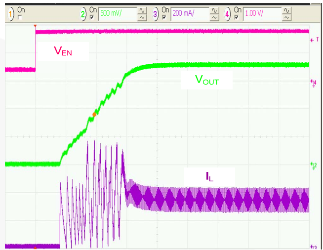
Figure 18. Soft-Start, R_{LOAD} = 6\Omega , 20 \mu s/div.
