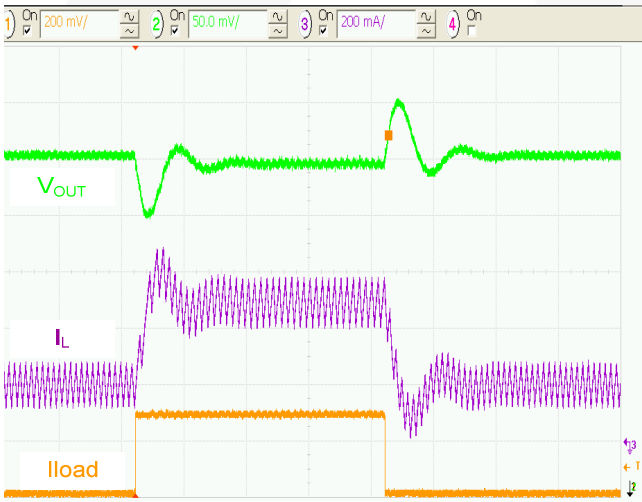
Figure 15. Load Transient 200 to 500mA, 3.6V IN , 5μs/div.
