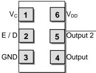
Terminations as viewed from the Top NOTE: XPRESSO LVDS VCXOs are designed to fit on Industry Standard, 6 pad layouts
