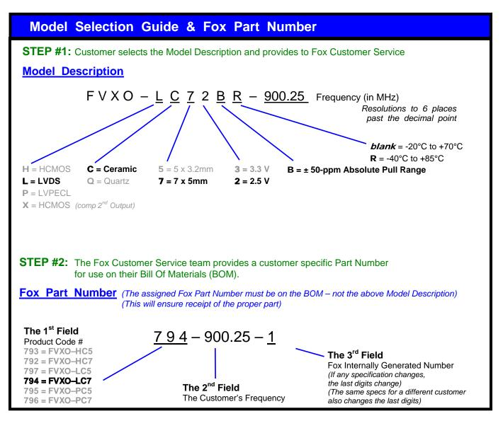
This example, FVXO-LC72BR-900.25 = Voltage Controlled, LVDS Output, Ceramic, 7 x 5mm Package, 2.5V, ±50 PPM Absolute Pull Range, -40 to +85°C Temperature Range, at 900.25 MHz
