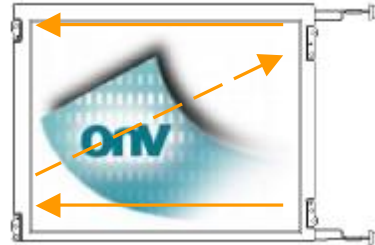
Fig. 2 Reverse scan (Pin19= High)
