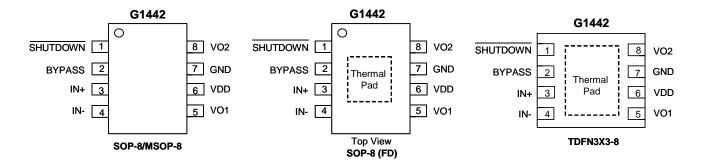
Note: Recommend connecting the Thermal Pad to the GND for excellent power dissipation.
