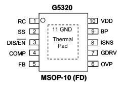
Note: Recommend connecting the Thermal Pad to the Ground for excellent power dissipation.
