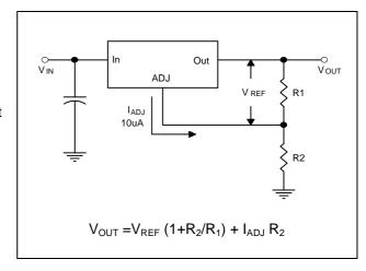
The power dissipation and junction temperature for H1085U in TO-263 package given by  $P_D=(V_{IN}-V_{OUT})\ I_{OUT},\ T_{JUNCTION}=T_{AMBIENT}+(P_Dx\theta_{JA}),\ Note:\ T_{JUNCTION}\ must not exceed 125°C$
