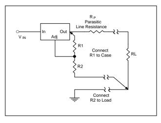
the top of  $R_1$  is internally connected to the output and ground pin can be connected to low side of the load as a negative side sense if, so desired.
