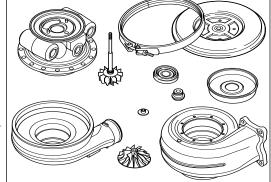
Soak the components in a non-corrosive low flash point metal cleaner to loosen deposits.
