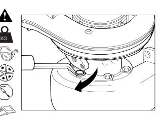
Following torque tightening it may be necessary to turn lockplate bolts in the tightening direction until a flat aligns with the lock tab. Use a hammer and drift to knock lockplate tabs into position against the turbine housing bolts.
