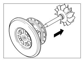
Carefully remove split ring seal, turbine (13) \* and discard.
