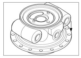
The speed sensor is designed to create an annular indentation in the bearing housing mating face to provide effective gas and oil sealing. With correct torque tightening, this face is re-useable and should appear clean and regular.
