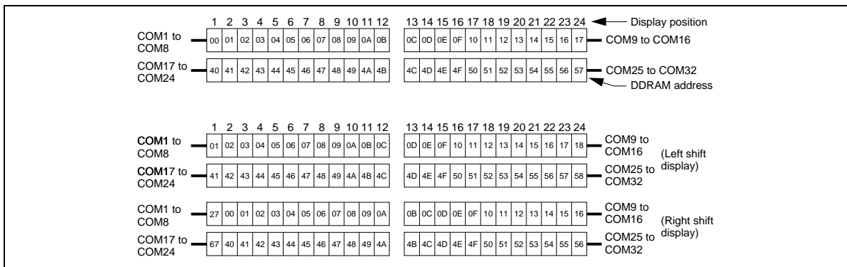
Figure 5 2-Line by 24-Character Display (5-Dot Font Width)
