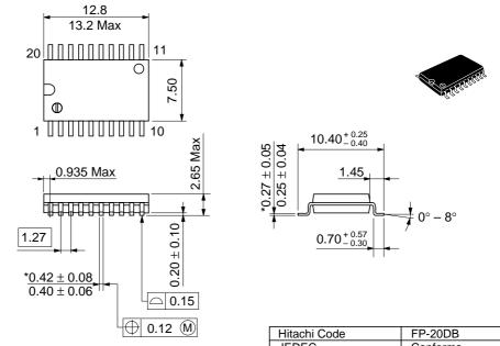
\*Dimension including the plating thickness Base material dimension
