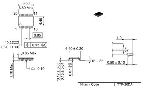
\*Dimension including the plating thickness Base material dimension
