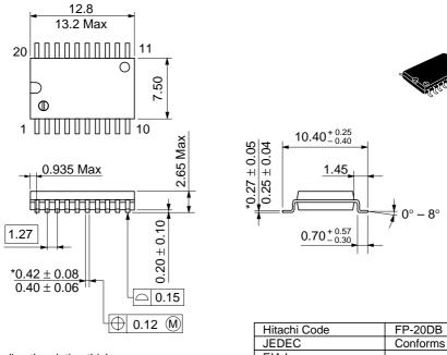
\*Dimension including the plating thickness
