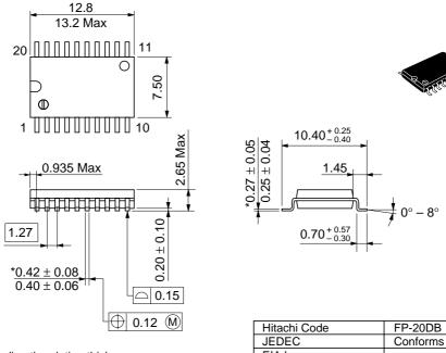
\*Dimension including the plating thickness
