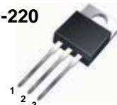
1.Gate 2. Drain 3. Source
