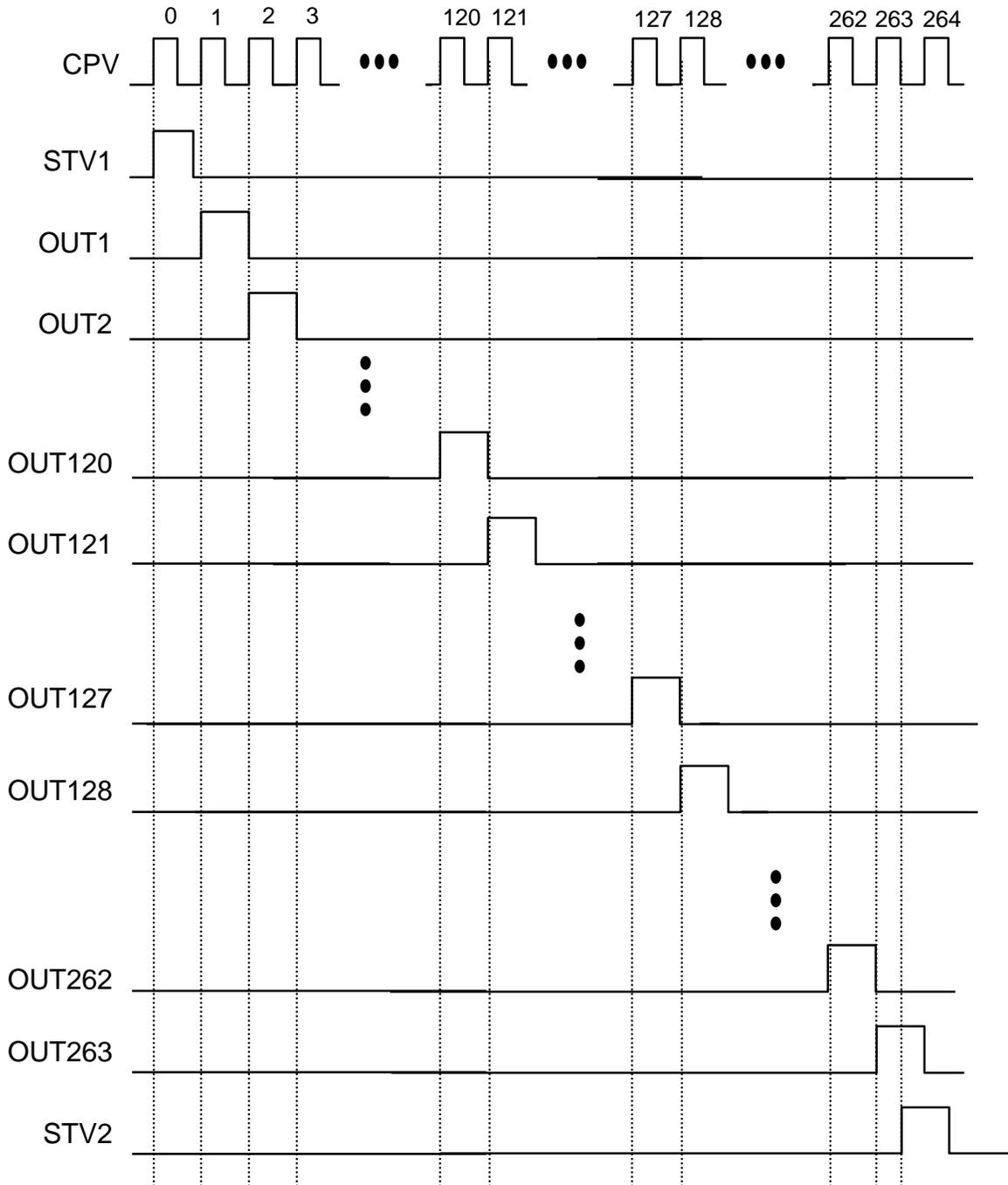
• **Timing Diagram ( When SDC = H, MODE = L )**
