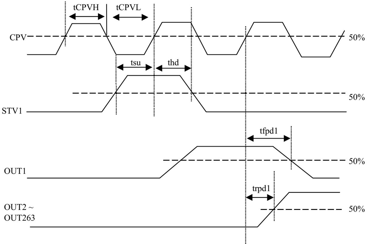
**•AC Characteristic Timing Diagram(2) (Where SDC=H)**
