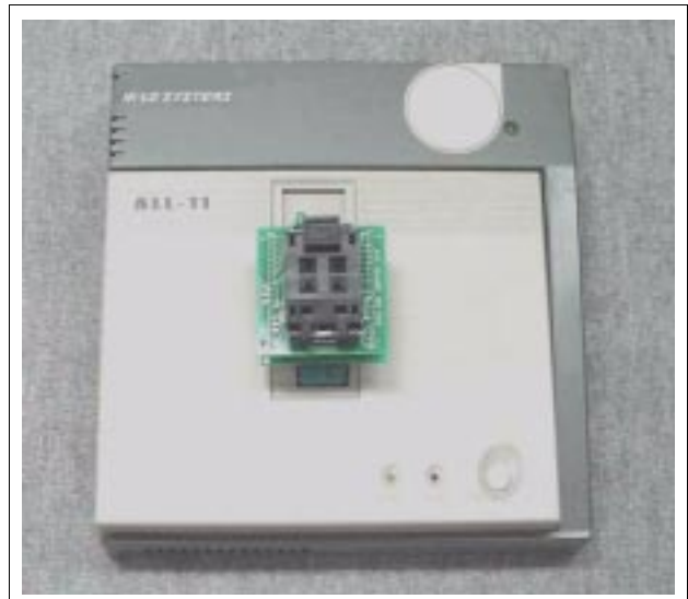
Figure 9-2 ALL-11 Programmer with adapter
