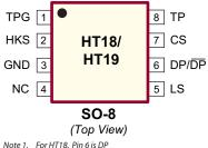
Note 1. For HT18, Pin 6 is DP For HT19, Pin 6 is  $\overline{DP}$
