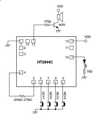
\* The IC substrate should be connected to VDD in the PCB layout artwork.
