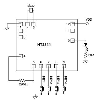
\* The IC substrate should be connected to VDD in the PCB layout artwork.
