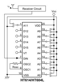
Note: Typical infrared receiver: PIC-12043T/PIC-12043C (KODENSHI CORP.) or LTM9052 (LITEON CORP.)
