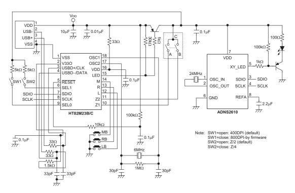
Note: Layout  $0.1\mu\text{F}$  capacitor,  $33\Omega$  resistor and  $0.01\mu\text{F}$  capacitor as close to VDD pin as possible.
