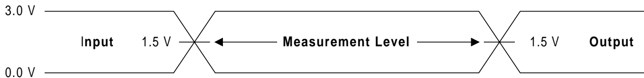
Figure 14. Input Waveforms and Measurement Levels
