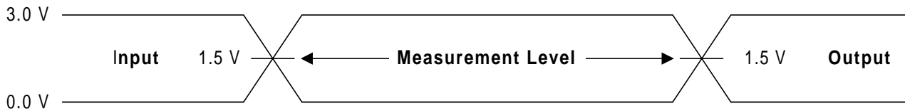
Figure 16. Input Waveforms and Measurement Levels
