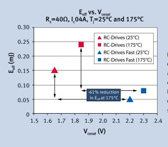
Due to differtent tradeoff between conduction and switching losses, either RC-Drives or RC-Drives Fast can be offered depending on switching frequency.
