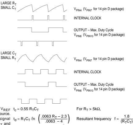
Oscillator timing capacitor  $C_T$  is charged by  $V_{REF}$  t<sub>c</sub>  $\approx 0.55 R_T C_T$ through  $R_T$  and discharged by an internal current source. During the discharge time, the internal clock signal blanks the output to the low state. Selection of  $R_T$  and  $C_T$  therefore determines both oscillator frequency and maximum duty cycle. Charge and discharge times are determined by the formulae:
