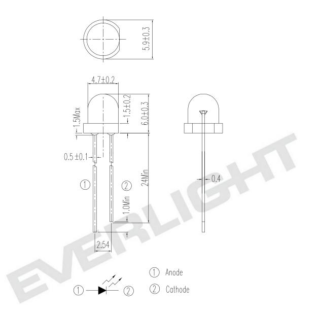
Note: Tolerances unless dimensions ±0.25mm
