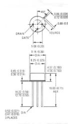
Conforms to JEDEC Outline TO-205AF (TO-39) Dimensions in Millimeters and (Inches)
