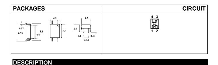
The IS357 is a single channel device suitable for use in vending machines, programmable controllers and copiers. The device incorporates an infra red LED and a phototransistor detector.
