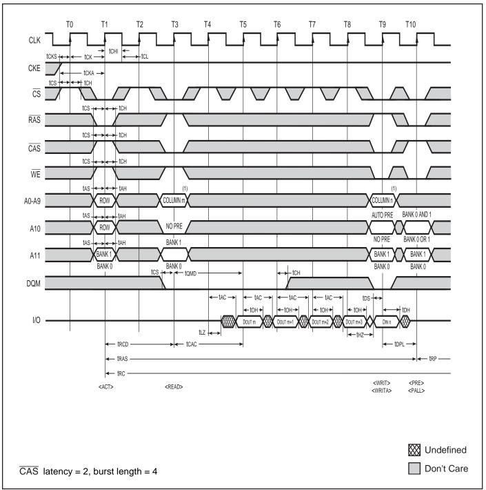
Read Cycle, Write Cycle / Burst Read, Single Write
