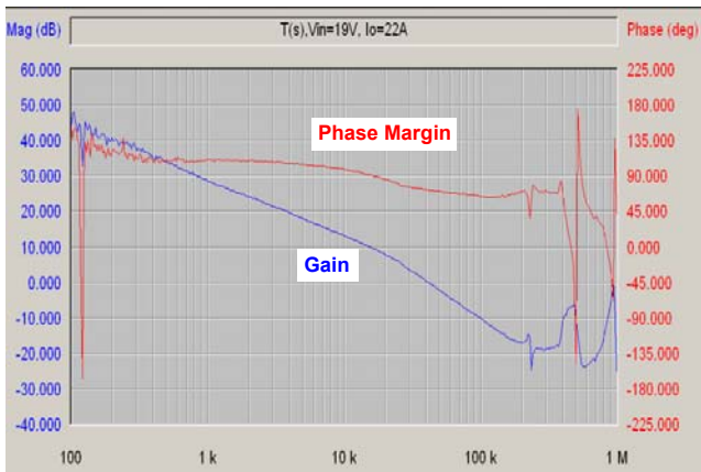
FIGURE 37. GPU MODE REFERENCE DESIGN LOOP GAIN T2(s) MEASUREMENT RESULT
