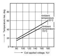
4. Ambient temperature characteristics (High capacity type)
