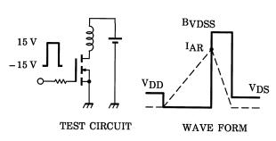
$$\begin{aligned} &RG = 25 \ \Omega \\ &V_{DD} = 90 \ V, \ L = 41 \ mH \end{aligned} \qquad E_{AS} = \frac{1}{2} \cdot L \cdot I^2 \cdot \left( \frac{BVDSS}{BVDSS - V_{DD}} \right)$$
