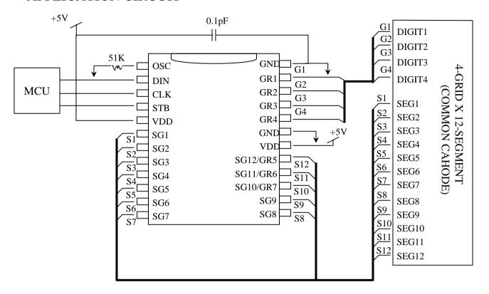
Note: The capacitor (0.1uF) connected between the GND and VDD Pins must be located as near as possible to the KK1207 chip.
