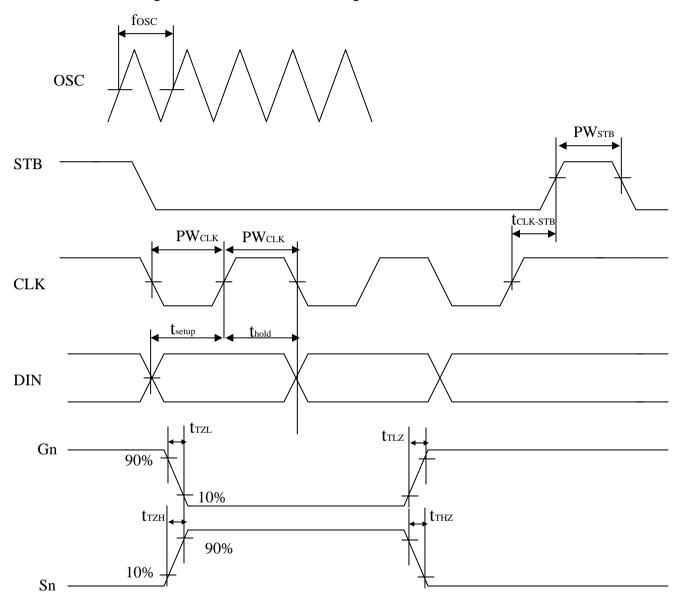
PW <sub>CLK</sub> (Clock Pulse Width)  $\geq$ 400ns t setup (Data Setup Time)  $\geq$  100ns t <sub>CLK-STB</sub> (Clock - Strobe Time)  $\geq$  1 $\mu$ s t <sub>TZL</sub> (Rise Time)  $\leq$  1 $\mu$ s t <sub>TZL</sub> <1 $\mu$ s
