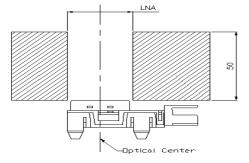
\*6: Maximum detection distance measuring method.
