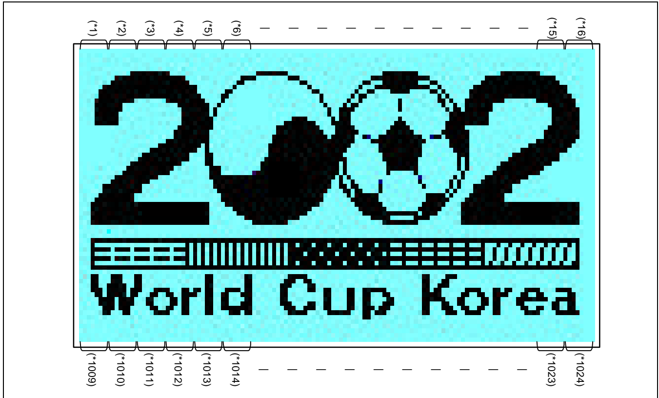
Figure 9. Relationship between CGRAM Full Graphic Mode Data Writing and Display Pattern (FG = "High")
