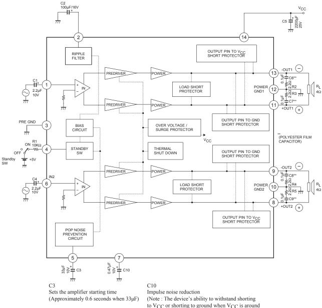
to  $V_{CC}$  or shorting to ground when  $V_{CC}$  is around 16V may be reduced as the value of this capacitor is increased. We recommend  $0.47 \mu F$ .)
