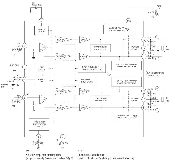
(Note : The device's ability to withstand shorting to  $V_{CC}$  or shorting to ground when  $V_{CC}$  is around 16V may be reduced as the value of this capacitor is increased. We recommend 0.47 $\mu$ F.)
