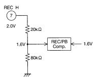
If the pin 7 DC voltage is < 2.0 V: Playback mode If the pin 7 DC voltage is > 2.0 V: Record mode H.Sync input: pin 6
