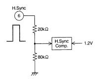
If the pin 6 DC voltage is > 1.5 V: Currently the signal is in an H.Sync period
