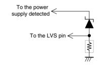
If the LVS pin is left open, the internal pull-down resistor will result in the IC seeing a ground level input, and the output will be turned off. Therefore, a voltage in excess of the LVS circuit clear voltage (about 4.4 V) must be applied to the LVS pin if the application does not use the undervoltage protection circuit. The maximum rating for the LVS pin applied voltage is 18 V.
