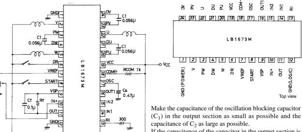
If the capacitance of the capacitor in the output section is large and the capacitance of C<sub>S</sub> is small, the starting votlage may rise at low temperatures. In 3V-use, reverse rotation of a motor would not be well, consider the resistance of Rcom.
