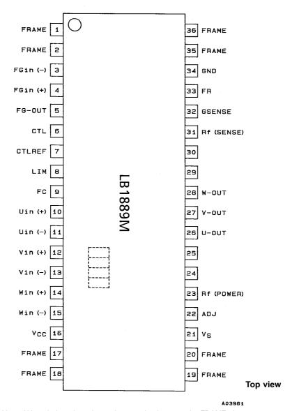
Note: Although there is no internal connection between the FRAME pin and GND, FRAME must be connected to GND externally for GND potential stabilization.
