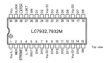
The package comes in two types-DIP30S and MFP30S.
