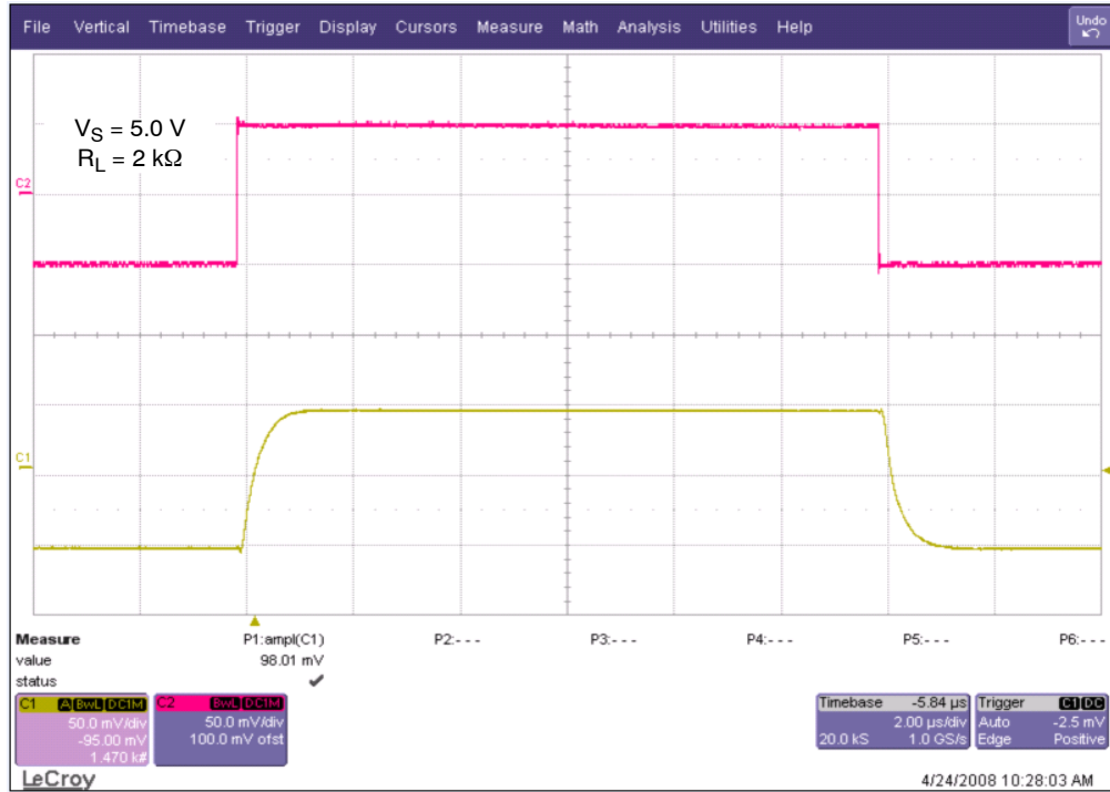
Figure 18. Small Signal Noninverting Response
