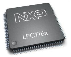
120 MHz, 32-bit Microcontrollers with Cortex-M3<sup>™</sup> core, LPC1700 series
