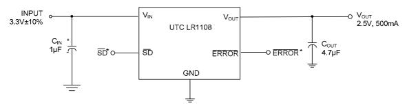
\* SD and ERROR pins must be pulled high through a 10kΩ pull-up resistor. Connect the ERROR pin to ground if this function is not used.
