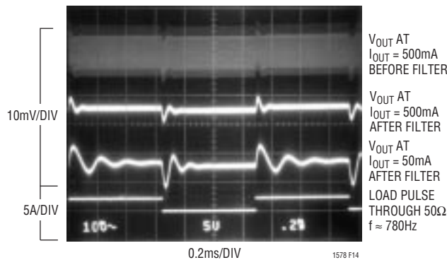
Figure 14. Loop Stability Check
