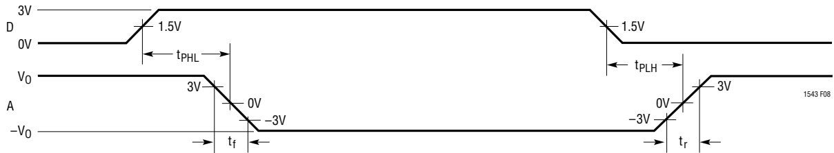
Figure 8. V.10, V.28 Driver Propagation Delays
