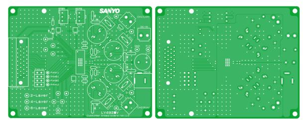
Mounted on a specified board (Customer bread board rev.1.0): 90.0mm × 70.0 mm × 1.6 mm (two-layer) Material: glass epoxy
