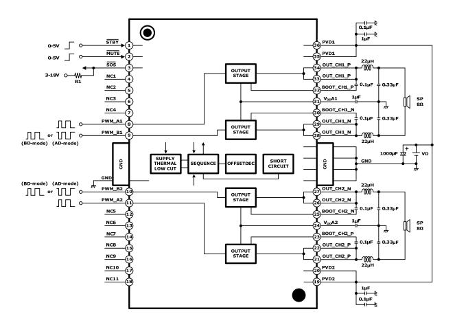
\*  $\overline{\text{SOS}}$  of pin 3 is the open collector output.
