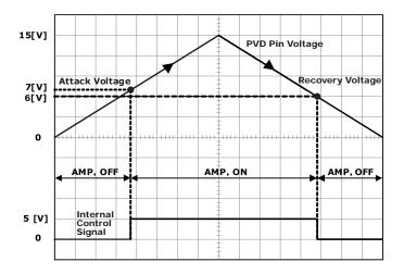
Output offset detection protection circuit
