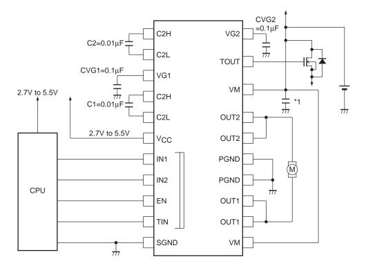
\*1 : Connect a kickback absorption capacitor directly near IC. Coil kick-back may cause rise of the voltage of VM line, and the voltage exceeding the maximum rating may be applied momentarily, resulting in deterioration or damage of IC.
