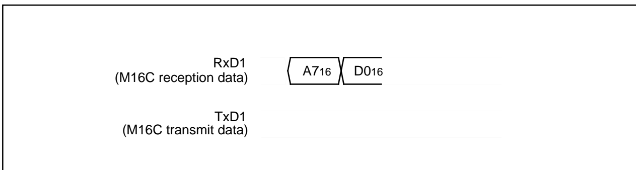
Figure 1.25.27. Timing for erasing all unlocked blocks
